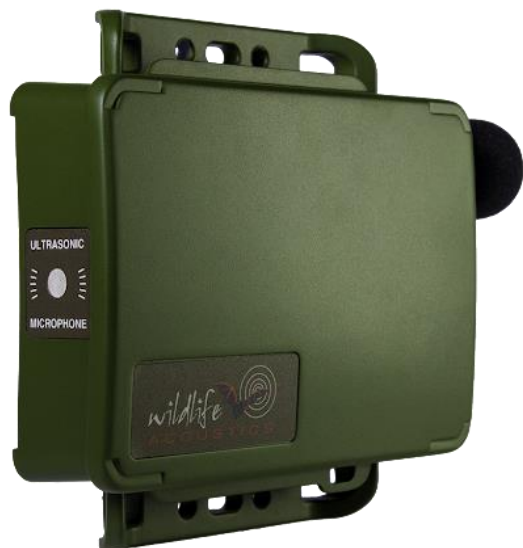
Figure 2. Song Meter Mini used to record low frequency sounds propagated by e-bikes and conventional bikes.
