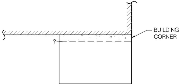
Footing = cement cobbles 3/8" to 4" diameter, locally cracked in many places, some roots growing into footing with/in soil in-filled cracks up to 1" wide
