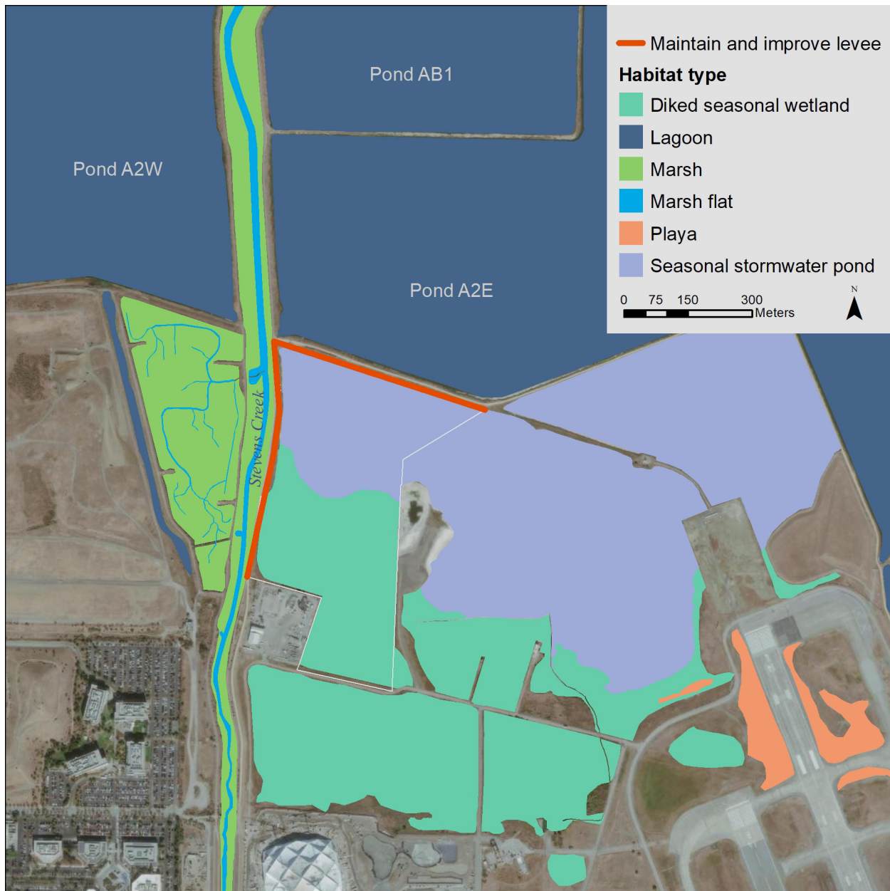
Figure 5.1. Option 1: Maintain existing diked marsh/stormwater pond
