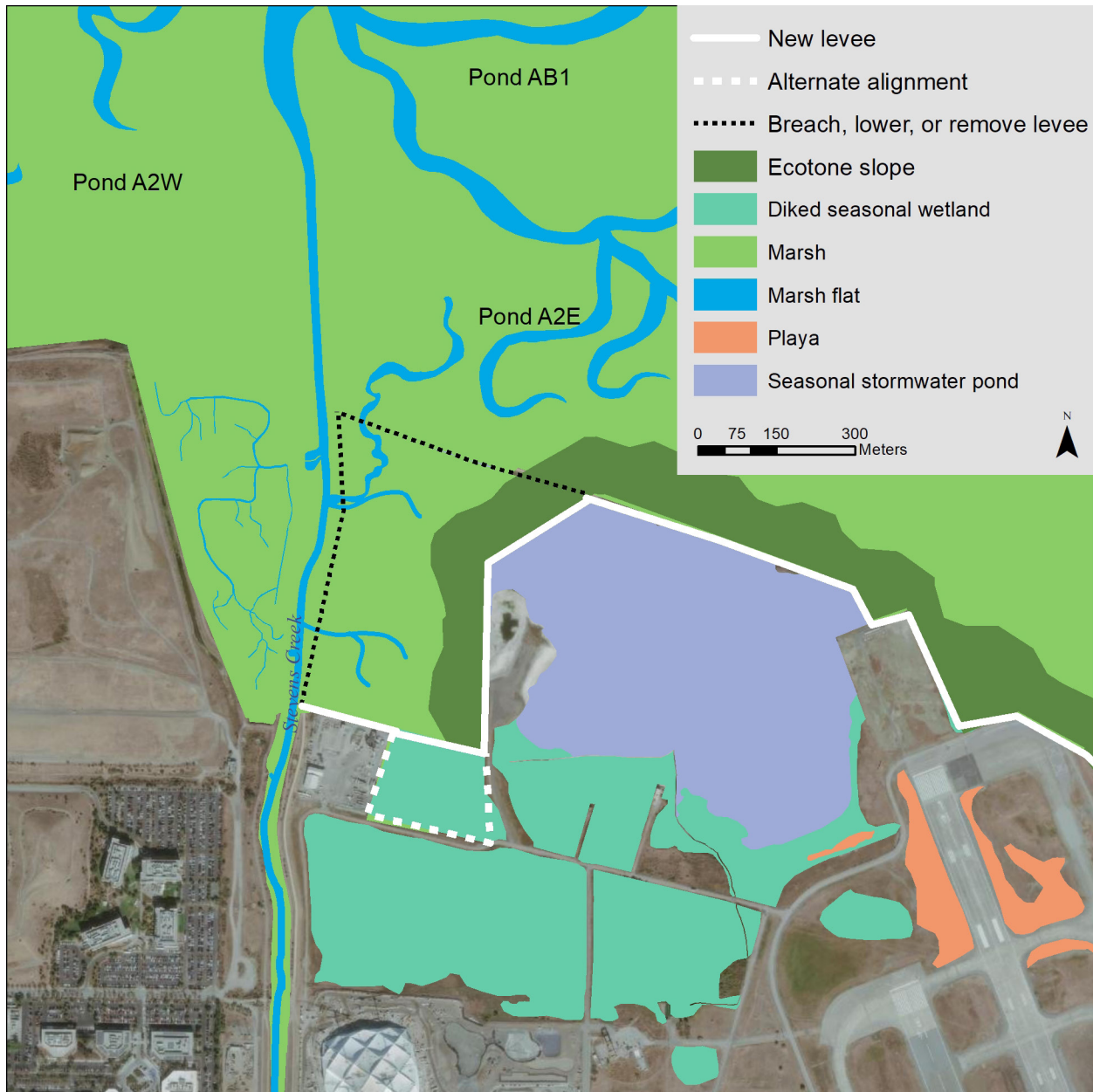
Figure 5.7. Option 4c: Restore full tidal action (salt ponds restored)
