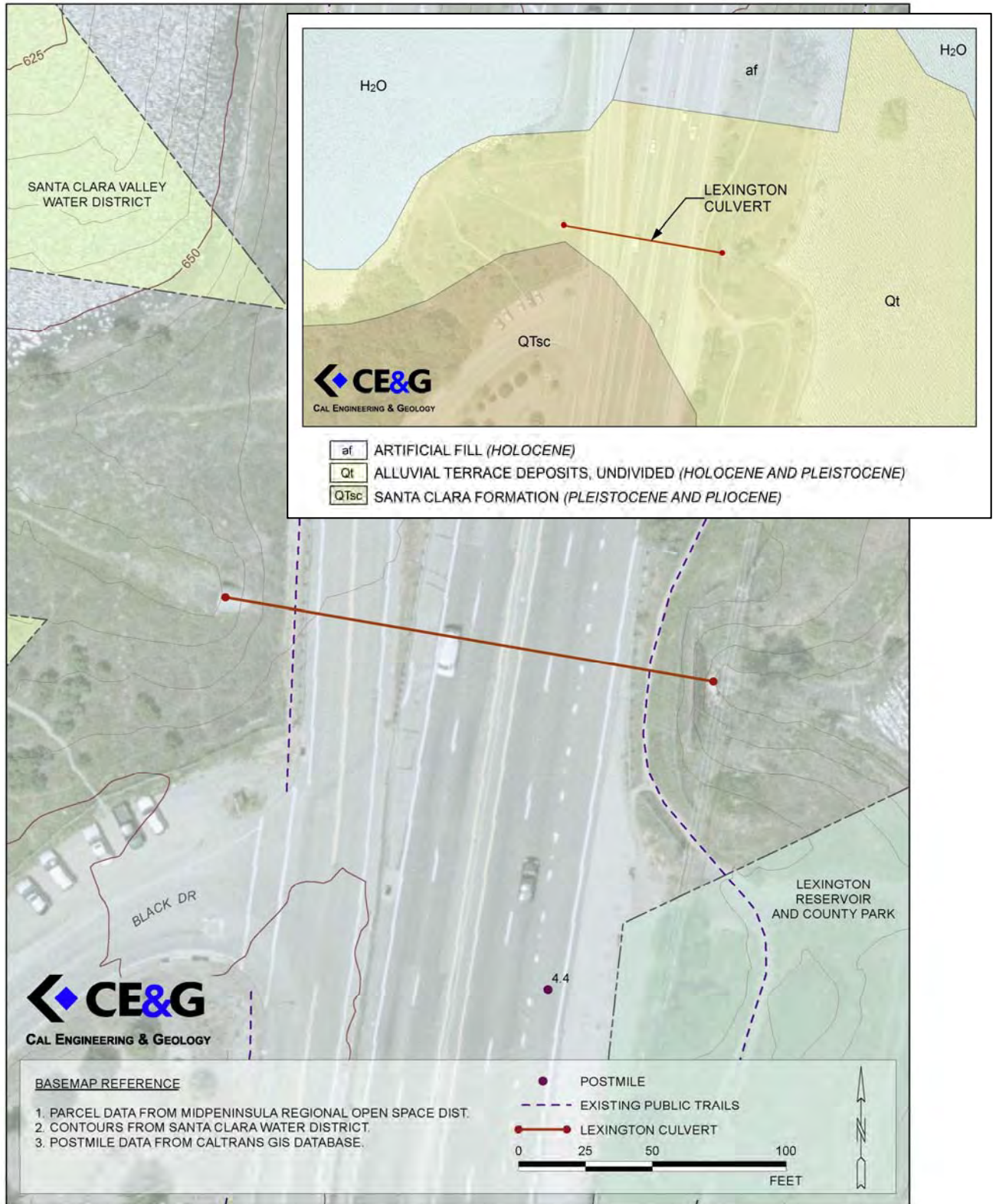
Figure 11: Lexington Culvert Site and Geology
