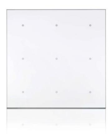
The AviProtek pattern 216 is a bird friendly solution with acid-etched visual markers on the exterior surface of the glass. This pattern is made with 6 mm dots spaced four inches apart in both the vertical and horizontal planes. This bird friendly pattern meets local regulations where dots spaced at four inches in both planes are accepted, such as in the city of Toronto, Canada (as of 2019).
