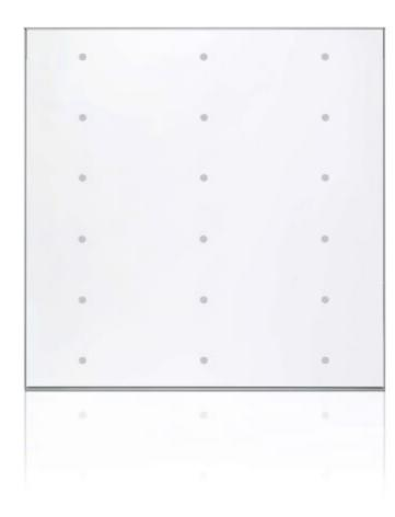
The AviProtek pattern 221 is a bird friendly solution with acid-etched visual markers on the exterior surface of the glass. The pattern is made with 5MM dots spaced two inches apart in the horizontal planes and four inches apart in the vertical planes. This pattern meets the recognized 2×4 rule as well as regulations or guidelines in municipalities where a bird friendly approach is required.
