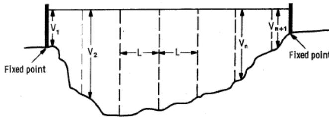
$$A = \frac{V_1 + 2V_2 + \dots + 2V_n + V_{n+1}}{2} \times L$$
