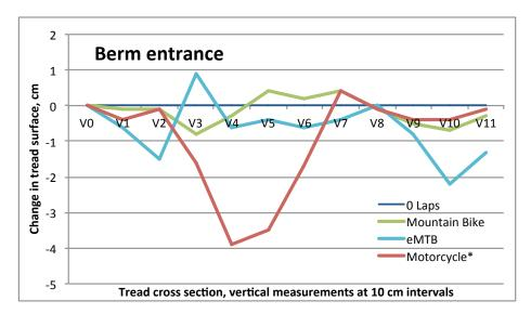
Figure 5. Trail profiles at 0 and 500 laps (0 and 200 for motorcycle). These show change in tread surface from the 0 lap measurement. Measurements taken at 10 cm intervals across each sample site, perpendicular to the trail. Greater soil displacement is seen for the Class 1 eMTB than for the mountain bicycle (some tread holes were observed forming), but much less than for the motorcycle. These are from comparable sample locations at the upper leg of a bermed turn.
