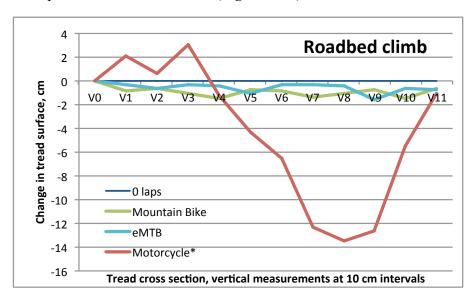
Figure 4. Trail profiles at 0 and 500 laps (200 laps for motorcycle). These show change in tread surface from the 0 lap measurement. For the motorcycle, you can see both trenching and piling of soil material as soil is displaced side-to-side and pushed downslope. These are from comparable sample sites on the roadbed.
