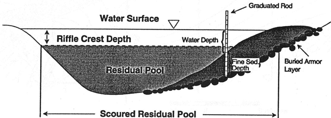
Figure 3-3 Sections of example pools illustrating the  $V^*$  method. Observers define the pool and riffle crest, set up a grid system of the longitudinal tape and transects, and perform sediment probing to measure the water depth and total depth to the bottom of finer sediment at approximately 100 points (from Hilton, S., and Lisle, T.E., 1993).
