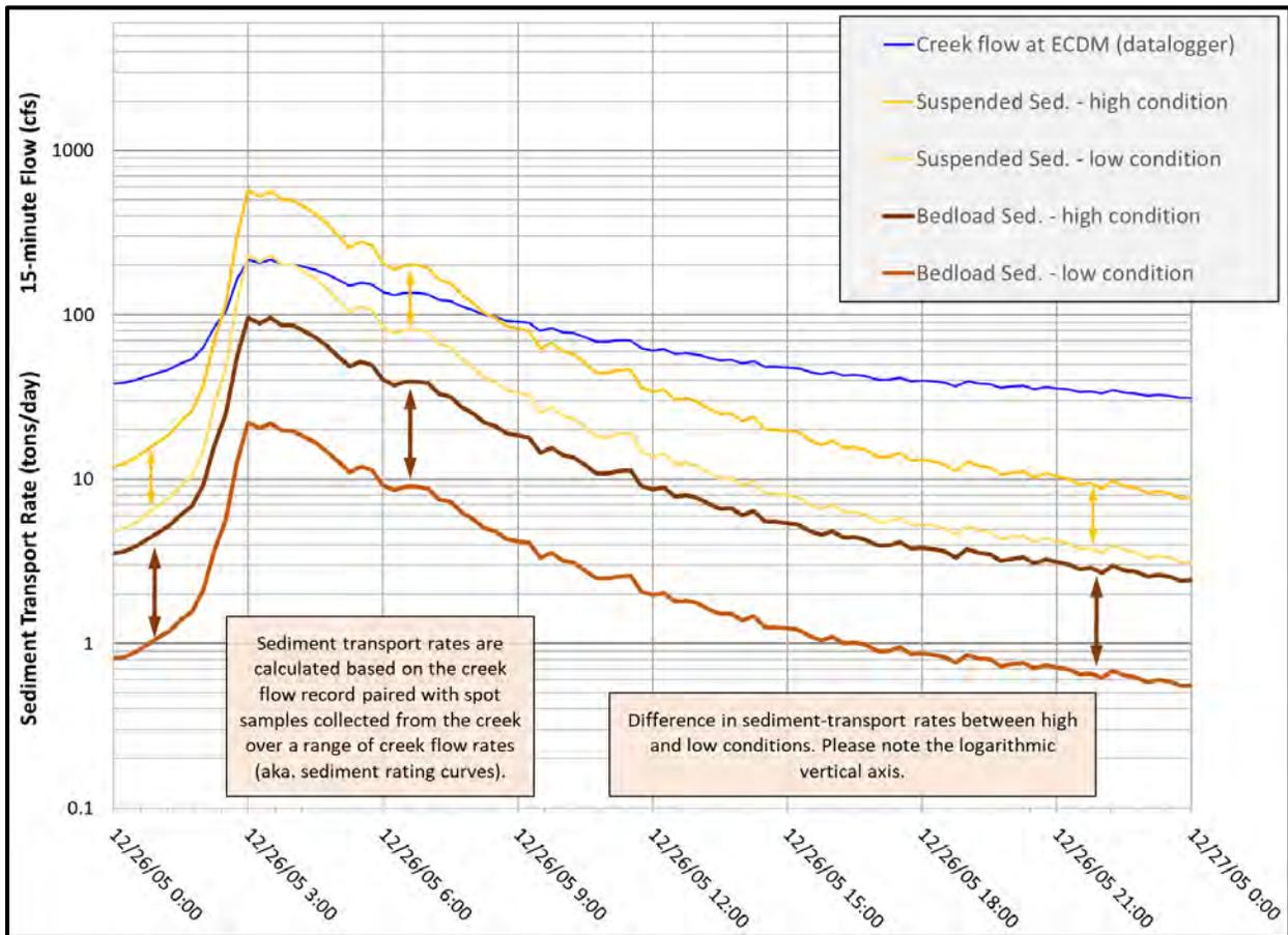
Figure 4-11 Sediment-transport rates during an example storm. In this example storm, the difference in sediment-transport rates between *high*- and *low*-sediment conditions are indicated by the arrows, for both bedload- and suspended-sediment rates.
