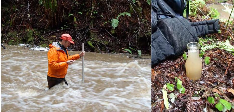
*Figure 4 Balance staff collecting sediment during a storm. Sample at right.*
