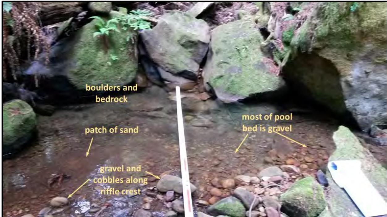
*Figure 5 Diagram Highlighting Stream Texture at a  $V^*$  pool*
