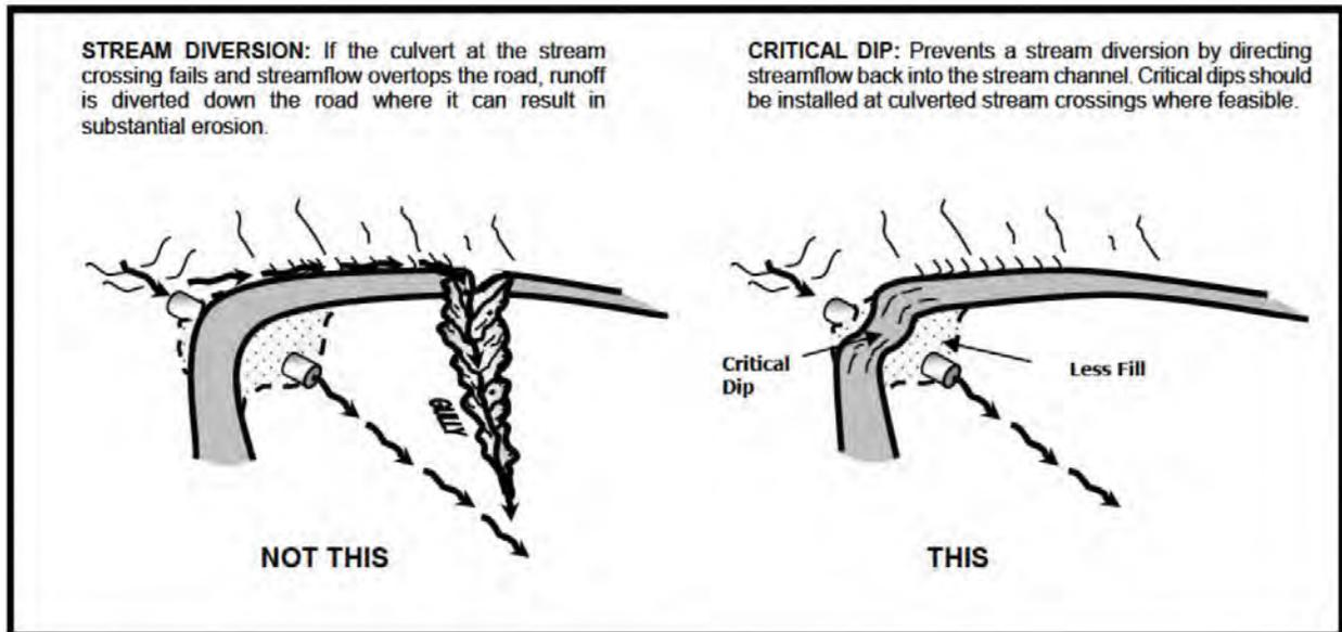
Figure 2-11 Typical sketch for using a critical dip with a culvert at a drainage/trail crossing. (from Best, 2002) A critical dip allows water to flow across the trail and back into the drainage, if the culvert were to become obstructed, rather than flowing along the trail for some distance.
