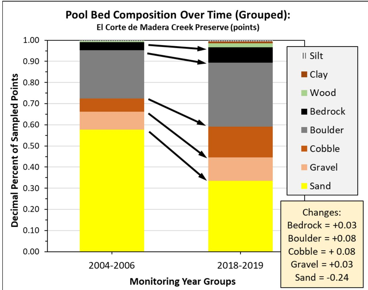
Figure 4-7 Change in grouped pool-bed composition from the start to the end of the WPP study; El Corte de Madera Creek Preserve. Percent of sand in pools decreased and other size classes increased, with percent of cobbles and boulders increasing the most.
