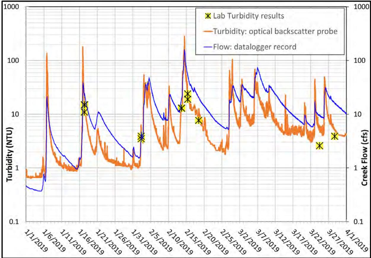
Figure 4-14 Turbidity record and hydrograph from water year 2019: El Corte de Madera Creek. Turbidity is low before storms, then rises quickly as creek flow rises, with the highest levels at the peaks of storm flow, and then declines following storms. Laboratory results of collected samples were used to adjust the sensor data. Values of 1 and 2 NTU look visibly clear.
