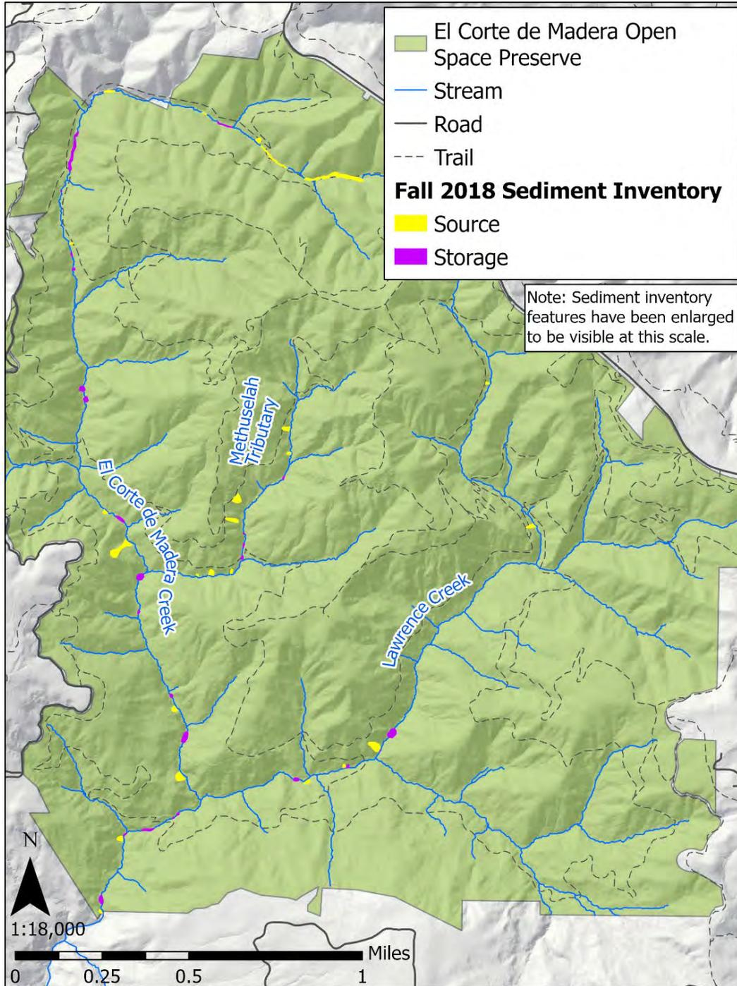
Figure 4-8 Map of large sediment sources and storage from 2018: El Corte de Madera Creek Preserve. Sediment sources are shown as yellow polygons, and storage areas are shown as purple. The sizes of polygons are exaggerated for graphical purposes, in order to be visible at this scale of map.
