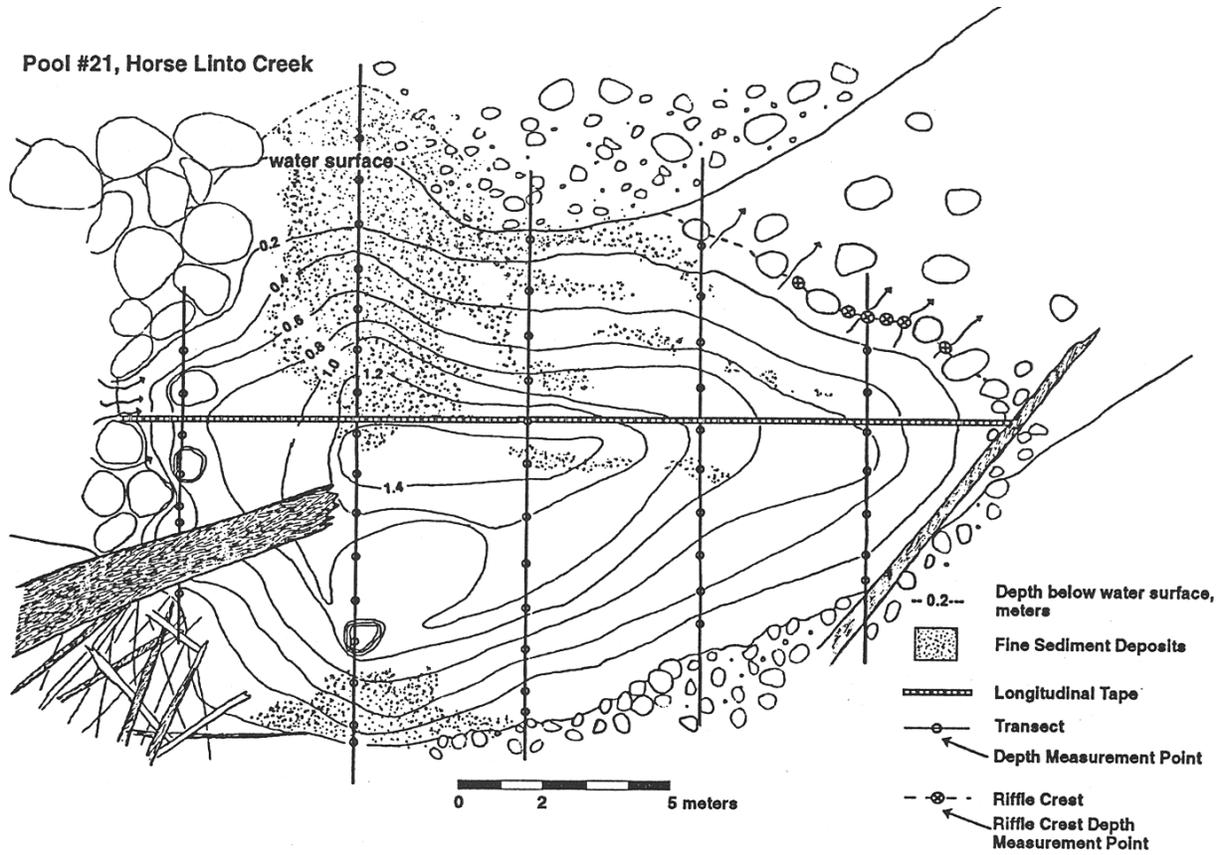
Figure 3-2 Plan View of an example pool to illustrate the V\* method. Observers define the pool, set up a grid system of the longitudinal tape and transects, and perform sediment probing to measure the water depth and total depth to the bottom of finer sediment (from Hilton, S., and Lisle, T.E., 1993).
