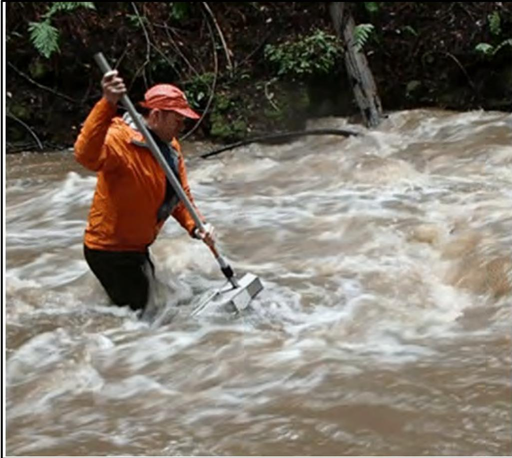
Figure 3-8 Bedload measurement near the peak flow of WY2018. We sampled bedload by wading across the creek and using a Helley-Smith bedload sampler at intervals across the active bed.
