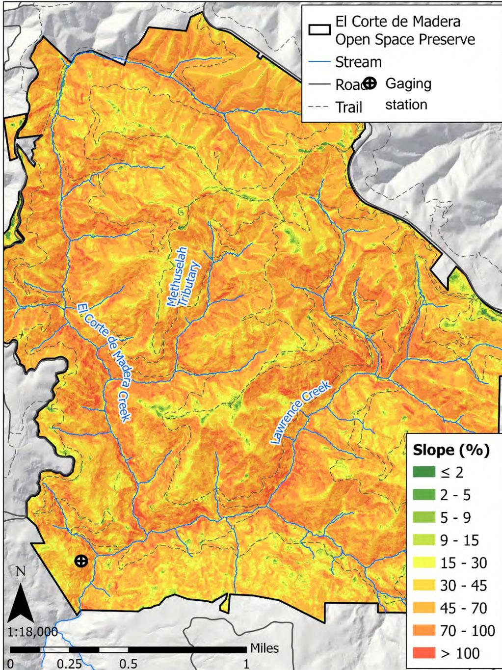
Figure 2-3 Slope steepness map analysis for El Corte de Madera Creek Open Space Preserve. Almost all the ECDM preserve consists of hillslopes of 15% or steeper, with most of the area having greater than 30% slopes; the steepest slopes are generally near the creek valleys. The area-averaged slope is 57% (30 degrees). (100% slope = 45 degrees)
