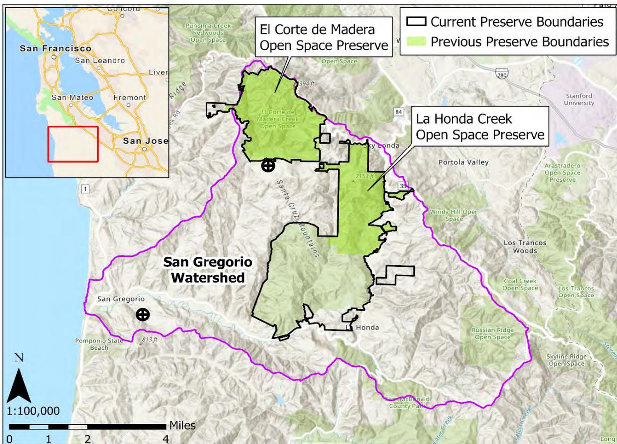
Figure 2-1 Regional and location map, with the larger San Gregorio Creek watershed delineated. The USGS and Balance Hydrologics creek gaging stations are shown. Skyline Boulevard (Route 35) runs along the northeast boundary of the Preserve. Highway 84 runs along the east side of the La Honda Creek Open Space Preserve.
