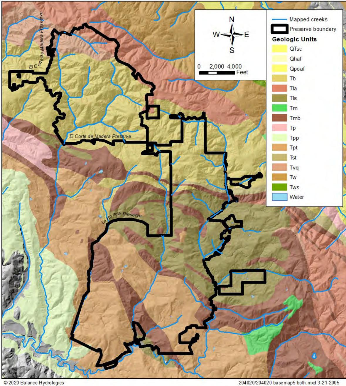
Figure 2-5 Geologic Map of the vicinity. The main geologic units are Butano (Tb) and Vaqueros (Tvq) sandstone. Some Mindego Basalt (Tmb) appears in the creek channel near the bottom of ECDM. The sandstone geology weathers to boulders, gravel, and sand-sized sediment. (Brabb, and Pampeyan, 1972, and Brabb, Graymer, and Jones, 1998)
