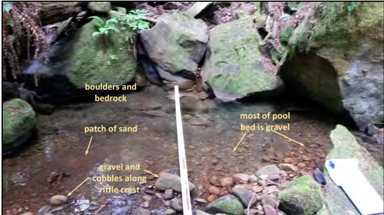
Figure 3-5 V\* pool showing different types of bed sediment that were recorded as part of the sediment-texture analysis. Photograph from 2018 when little sand was on the bed; the V\* value of this pool was measured to be 0.13 at the time.
