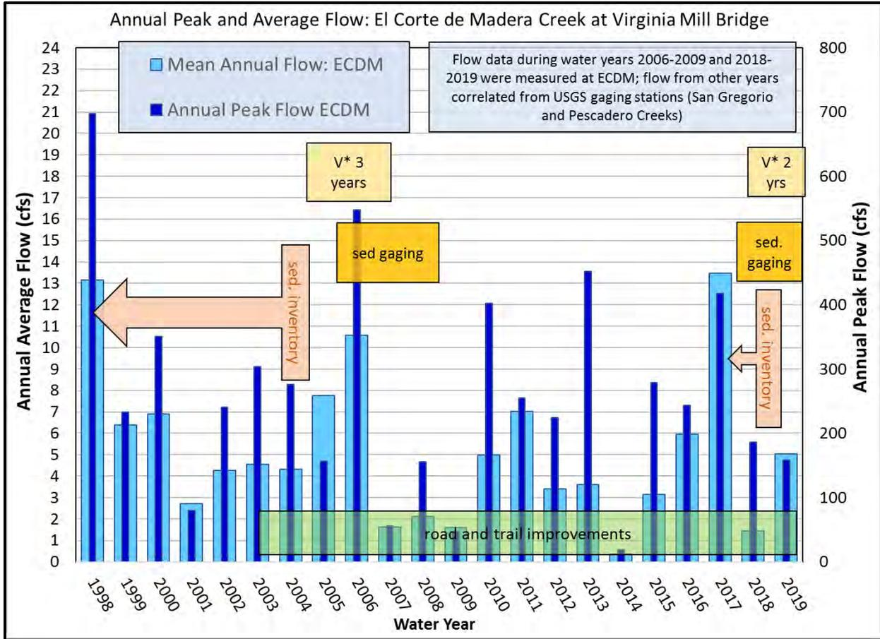
Figure 3-1 Periods of measurement approaches overlaid with a chronological plot of average annual flow and annual peak flow. The sediment inventory looks back several years to when landslides and bank collapses occurred (1998 and 2017). Water year 2006 was also a disruptive year in terms of the peak flow and bed changes, which overlapped with the V\* measurements and flow and sediment gaging.
