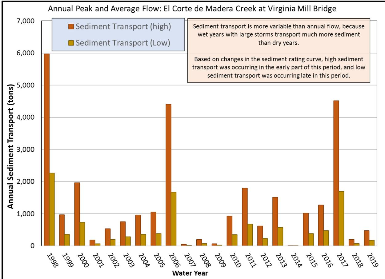
Figure 4-16 Calculated annual sediment transport: El Corte de Madera Creek at Virginia Mill bridge. Sediment transport is more variable than annual flow, because wet years with large storms transport much more sediment than dry years. Based on changes in the sediment rating curve, high sediment transport was occurring in the early part of this period, and low sediment transport was occurring late in this period.
