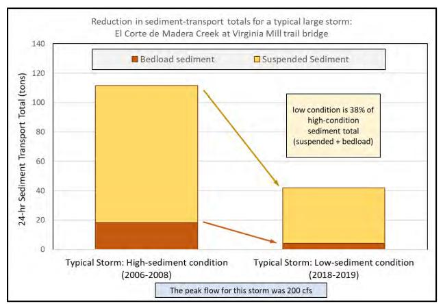
Figure 4-10 Reduction in the amount of sediment transported during a typical large storm. For this storm hydrograph, the amount of sediment transported now would be 38% of the sediment transported during the first sampling period. The 24-hour flow record used for this calculation occurred December 26, 2005. A storm peak of 200 cfs equates to a 1.6-year storm.
