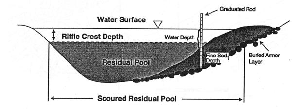
Figure 3-3 Sections of example pools illustrating the V\* method. Observers define the pool and riffle crest, set up a grid system of the longitudinal tape and transects, and perform sediment probing to measure the water depth and total depth to the bottom of finer sediment at approximately 100 points (from Hilton, S., and Lisle, T.E., 1993).
