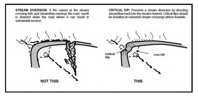
Figure 2-11 Typical sketch for using a critical dip with a culvert at a drainage/trail crossing. (from Best, 2002) A critical dip allows water to flow across the trail and back into the drainage, if the culvert were to become obstructed, rather than flowing along the trail for some distance.
