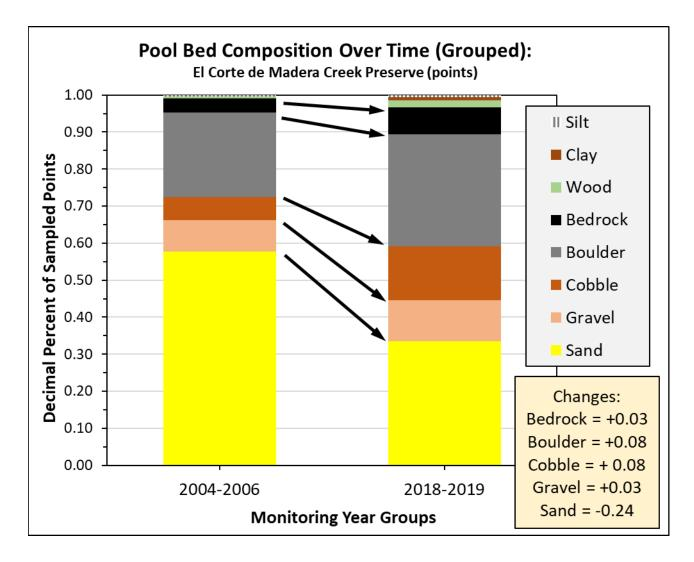
Figure 4-7 Change in grouped pool-bed composition from the start to the end of the WPP study; El Corte de Madera Creek Preserve. Percent of sand in pools decreased and other size classes increased, with percent of cobbles and boulders increasing the most.
