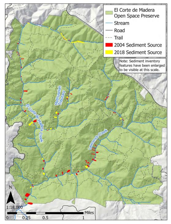
Figure 4-9 Map of large sediment sources inventoried in 2004 and again in 2018. Sediment sources from 2004 are shown as red polygons, and those from 2018 are shown as yellow. The sizes of polygons are exaggerated for graphical purposes in order to be visible at this scale of map.
