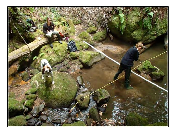
Figure 3-4 V\* measurements being performed by MROSD interns: El Corte de Madera Creek Preserve, 2019. The downstream end of the pool (riffle crest) was defined here at approximately 3 feet on the tape, where the small boulders separate the flat pool surface from the moving water surface. The dog was a "volunteer" who had wandered into the Preserve, and was reunited with his owners- with assistance from MROSD rangers- at the end of the day (dogs are not permitted in ECDM).
