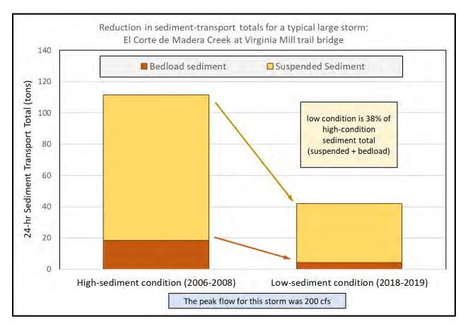
Figure 7 A 1.6-year storm event transporting sediment out of ECDM, comparing the before and after conditions.
