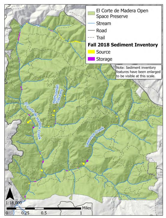
Figure 4-8 Map of large sediment sources and storage from 2018: El Corte de Madera Creek Preserve. Sediment sources are shown as yellow polygons, and storage areas are shown as purple. The sizes of polygons are exaggerated for graphical purposes, in order to be visible at this scale of map.
