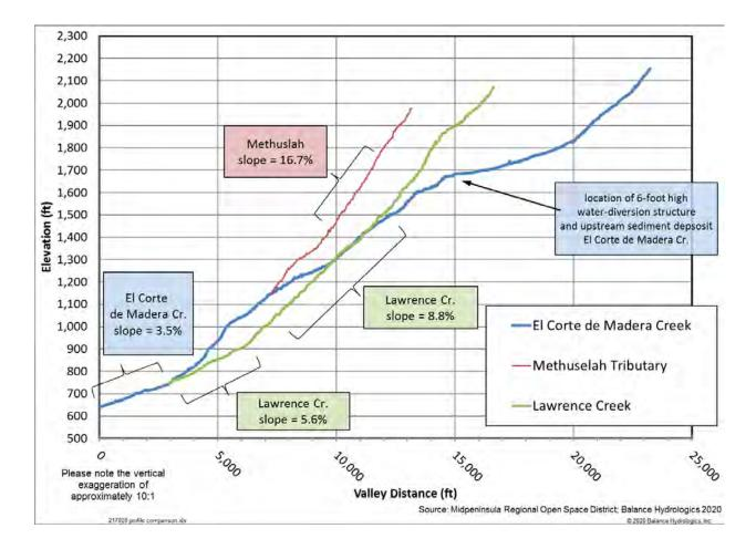
Figure 2-4 Creek valley slopes for El Corte de Madera Creek, Lawrence Creek, and the designated Methuslah tributary: El Corte de Madera Creek Preserve. The changes in slope along El Corte de Madera Creek are likely mainly geologic in origin. The creek profiles diverge at their confluences. Creek valley slope will typically be steeper than the local creek slope, because the valley slope calculation does not fully account for meanders and smaller scale twists and turns in the creek channel.
