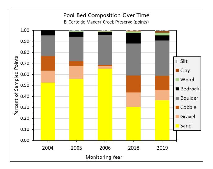
Figure 4-6 Change in pool bed material over time (by measurement point): El Corte de Madera Creek Preserve. This plot shows that the occurrence of sand in pool bottoms decreased from the 2004-2006 monitoring period to the 2018-2019 monitoring period, and that cobbles and boulders increased. These results largely mirror the V\* results. This plot also shows that the two main sediment sizes in pools are boulders and sand.
