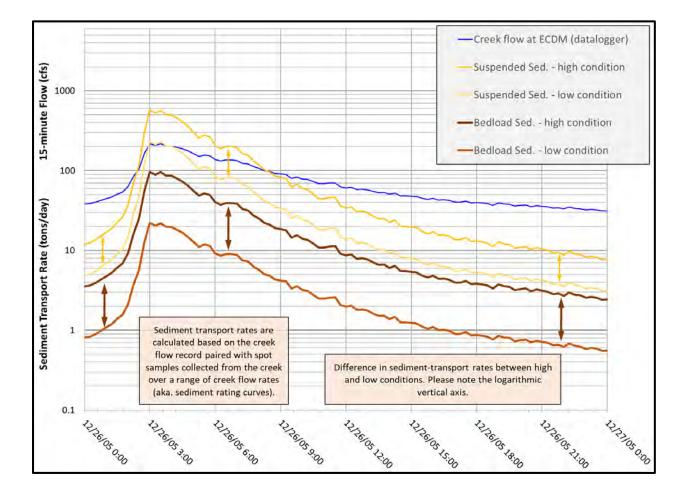
Figure 4-11 Sediment-transport rates during an example storm. In this example storm, the difference in sediment-transport rates between *high*- and *low*-sediment conditions are indicated by the arrows, for both bedload- and suspended-sediment rates.
