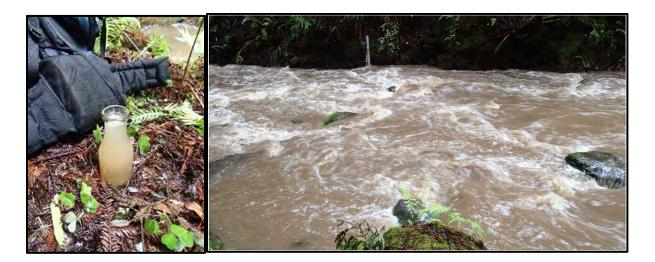
Figure 3-7 Sample in collection bottle and typical conditions during moderate to high flow: El Corte de Madera Creek at gaging station. Water is turbid and well mixed. We collected width- and depth-integrated suspendedsediment samples with a DH-48 sampler that we then analyzed for turbidity and suspended-sediment concentration.
