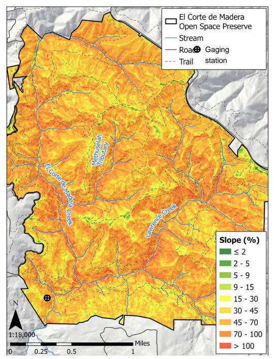
Figure 2-3 Slope steepness map analysis for El Corte de Madera Creek Open Space Preserve. Almost all the ECDM preserve consists of hillslopes of 15% or steeper, with most of the area having greater than 30% slopes; the steepest slopes are generally near the creek valleys. The area-averaged slope is 57% (30 degrees). (100% slope = 45 degrees)
