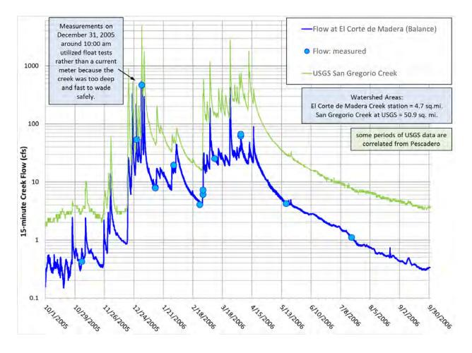
Figure 2-7 Flow hydrograph recorded for water year 2006: El Corte de Madera Creek at Virginia Mill bridge. Water year 2006 was a wet year with several large storms; the largest occurred December 31, 2005, with a peak flow of 548 cfs (which equates to roughly a 13-year storm).
