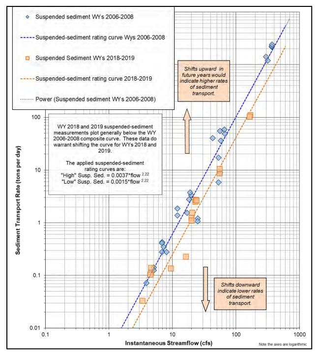
Figure 4-12 Suspended-sediment transport measurements and rating curve: El Corte de Madera Creek at Virginia Mill Trail. Blue symbols are samples collected during water year 2006 through 2008; orange symbols are sample collected during water years 2018 and 2019. Suspended-sediment sampling indicates that there has been a noticeable decrease in the amount of suspended sediment entrained over the range of flow.
