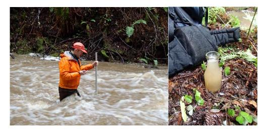
*Figure 4 Balance staff collecting sediment during a storm. Sample at right.*
