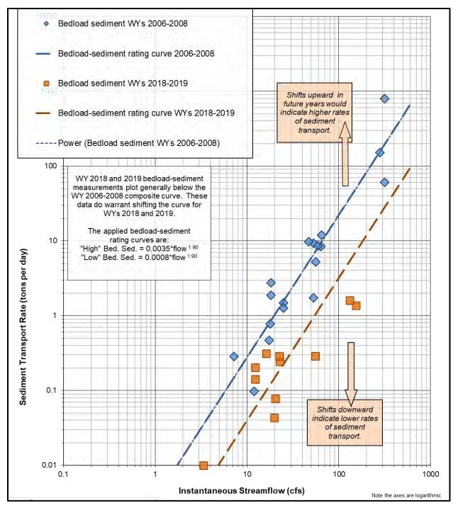
Figure 4-13 Bedload-sediment transport measurements and rating curve: El Corte de Madera Creek at Virginia Mill Trail. Blue symbols are samples collected during water year 2006 through 2008; orange symbols are sample collected during water years 2018 and 2019. Bedload-sediment sampling indicates that there has been a noticeable decrease in the amount of suspended sediment entrained over the range of flow.
