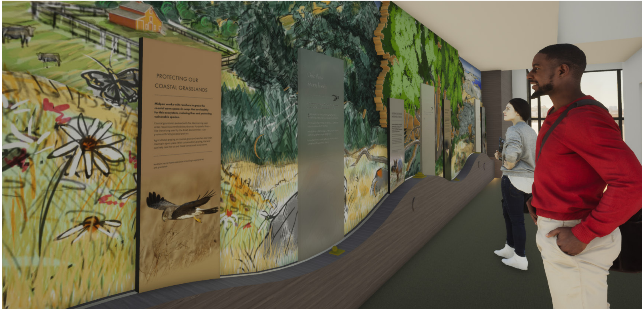
Detail of exhibit wall showing layering of illustrated mural on appleplywood with graphic panels in front. A subtle band of lighting shines up onto the mural from the top edge of the redwood band below. On top of redwood band will be a ribbon of graphics identifying species and preserves. Tactile elements are perched on top of the redwood band.
