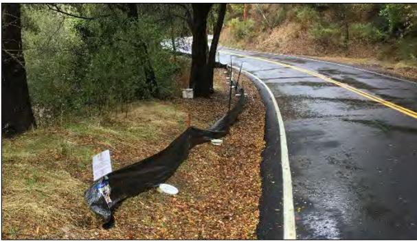
**Photo 3.** Array V showing pairs of traps on the upslope and downslope side of the array.
