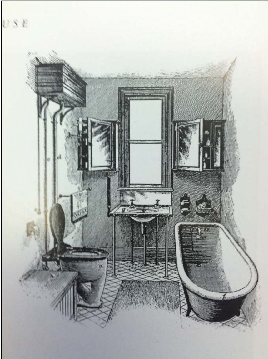
A rendering of a Victorian-era bathroom as illustrated in Randolph Delehanty's book In the Victorian Style. This bathroom has very similar fixtures to those in Hawthorn House, including the standing lavatory with counter and cast iron tub.
