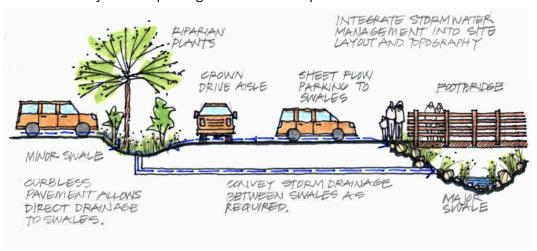
10. Integrate stormwater systems into site grading.
