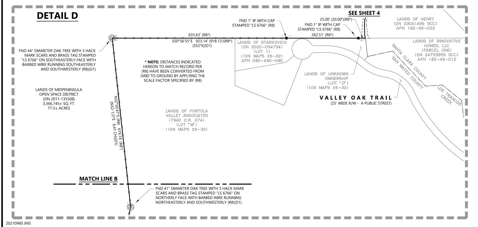
FND 41" DIAMETER OAK TREE WITH 3 HACK MARK SCARS AND BRASS TAG STAMPED "LS 6766" ON NORTHERLY FACE WITH BARBED WIRE RUNNING NORTHEASTERLY AND SOUTHWESTERLY (R8)(D1) SFNF - CHAMFERED FENCE POST (D1)(R2)(R4)(R5) HELD RECORD ANGLE AND DISTANCES FROM
