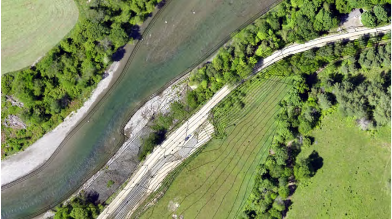
Figure 9 Riverside Image with Topography Represented in Three-Dimensions as Captured Using an UAV
