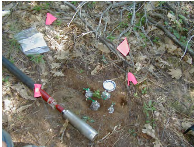
Figure 10 Soil Sample Plot Showing Soil Corer, temperature, and in this Photo, Nitrogen Sampling Bags
